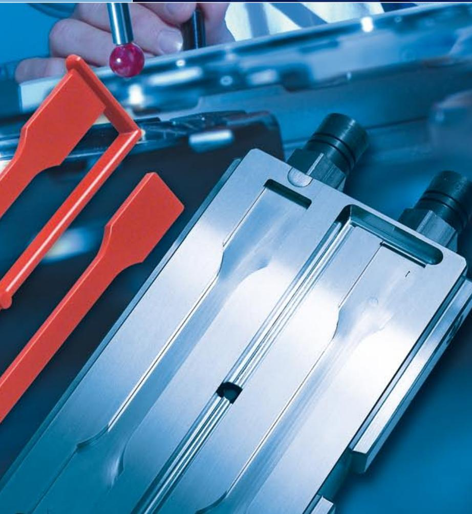
**A modular concept.** The modular AIM Mould System comprises a mould base, a mirror plate and as many product-forming inserts as you require. Mould bases, mirror plates and standard ISO inserts are delivered 'off the shelf'. Inserts for other standards are delivered within a matter of weeks.
